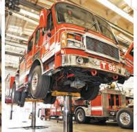
At the central Fire Supply and Maintenance Yard, the LAFD uses 23 vehicle lifts. Most are two-piston; the lift in this photo is a triple piston, one of the largest the City uses. The lift can handle up to 20,000 pounds. These lifts are eco-friendly and hydraulic, with one motor for each lift piston.
