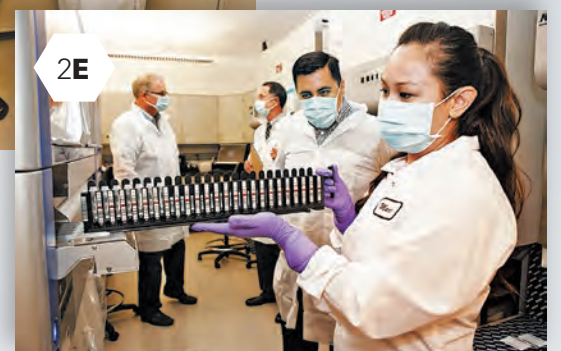
Martie Donnelly inserts trays of evidence into the QIASymphony extraction machine. In generally two to three hours, the extraction process will be completed on this batch.
