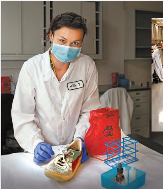
Alla Tashmukhamedova, Criminalist II, 3 years of City service, uses a swab to sample a small portion of a red stain on this shoe. She will then apply phenolphthalein to the swab, and look for a color change. Phenolphthalein turns pink when it comes in contact with blood.
