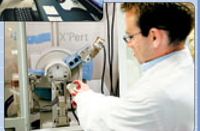
BELOW: Matt Franzman inserts the chemical or material in question into the X-ray diffractometer, which scans the material.
