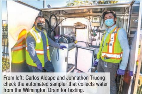
From left: Carlos Aldape and Johnathon Truong check the automated sampler that collects water from the Wilmington Drain for testing.
