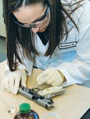
works on restoring a gun's serial number (actual casework)
