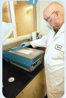
In this demonstration (not actual casework), a "blank" sheet is placed on the top of the ESDA machine.
