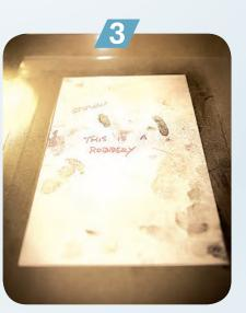
The toner highlights the indentations, and examiners can then read what was written on the top sheet of the pad. This process can also reveal fingerprints, which the Questioned Documents Unit passes along to the Latent Print Unit for processing. (This sheet is for demonstration purposes only and is not actual casework.)
