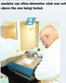
the sheet of paper to protect the evidence. The sheet is made smooth with a roller. With the machine on, air pulls the sheet to the bed, and a slight electrostatic charge is given to the sheet. Then, a special toner is poured on top of the blank sheet (covered
