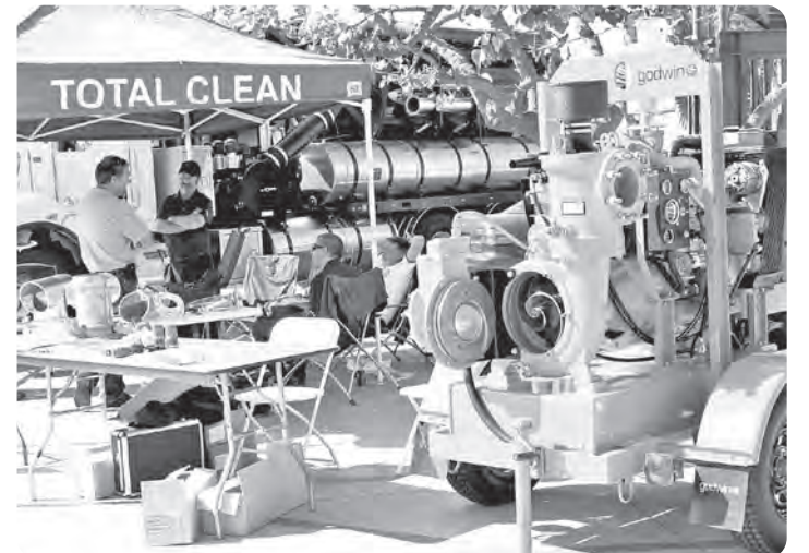
One of the pieces of collection equipment on display is a transfer pump, used to bypass sewers and pump water and debris.
