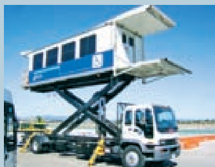
This ADA-compliant bus reaches high to sit parallel with a plane's exit doors, helping disabled passengers deplane safely and efficiently.
